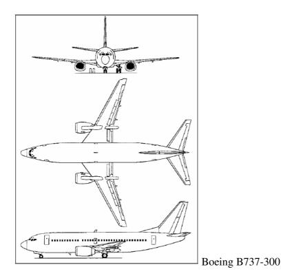
**Conventional aircraft configurations** all have one fuselage, one wing, and an empennage at their rear end. This configuration is also called *tail aft aircraft*.
