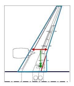
A **kinked wing** trailing edge provides space for the integration of a wing mounted landing gear in case of an aft swept wing. The main landing gear is positioned aft of the center of gravity. Also the wing is positioned with respect of the center of gravity.
