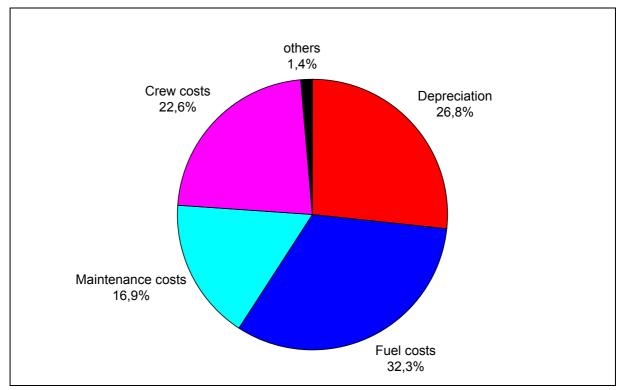
**Fig. 14.6** Direct Operating Costs (DOC) of the Boeing 767 from Fig. 14.5. A common way of presentation of DOC is the pie chart
