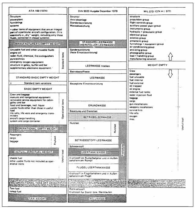
Fig. 10.2: Comparison of mass breakdowns according to [ATA 100], [DIN 9020] and MIL-STD-1374. Source: [DIN 9020]
