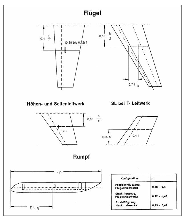
**Fig. 10.8:** The position of the centers of gravity of mass groups according to [MARCKWARDT 98a] based on data from [TORENBEEK 88]
