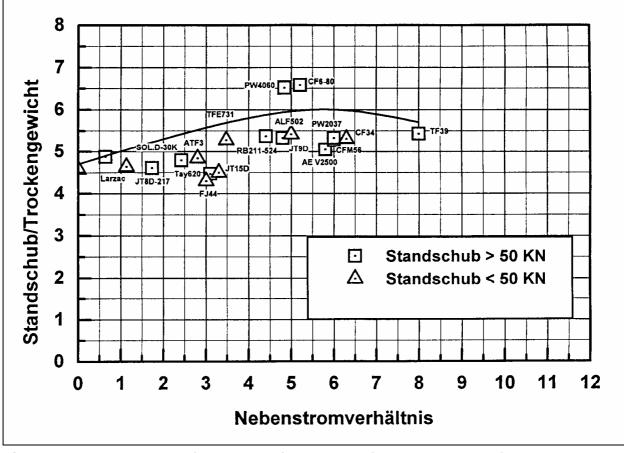
**Fig 10.5:** Estimate of mass  $m_E$  of jet engines [MARCKWARDT 98a]
