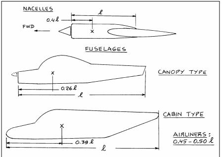
Fig. 10.7: The position of the centers of gravity of mass groups according to [ROSKAM II] based on data from [TORENBEEK 88]
