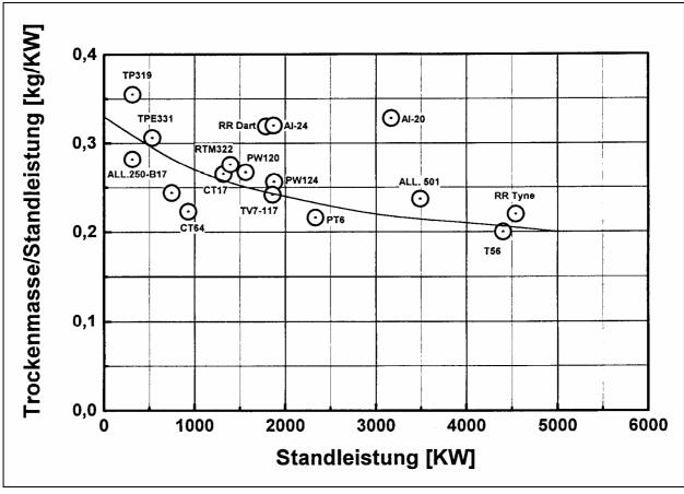
Fig. 10.6: Estimate of mass  $m_E$  of turbo prop engines [MARCKWARDT 98a]
