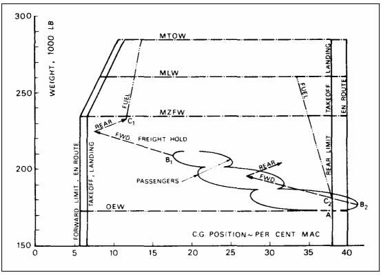
Fig. 10.9: Load and trim sheet [TORENBEEK 88]
